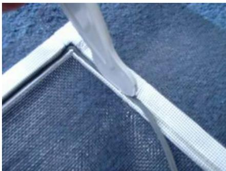
2. Lay the assembled frame on a flat surface with the inner groove facing you. Place the mesh over the panel and start to push the rubber gasket into the groove using the tool supplied. Trim off any excess mesh with a sharp Stanley knife.
