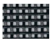
Construction - fibreglass / PVC ultrasonically welded
