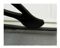
3. Lay the assembled frame on a flat surface with the inner groove facing you. Place the mesh over the panel and start to push the rubber gasket into the groove using the tool supplied. Trim off any excess mesh with a sharp Stanley knife.
