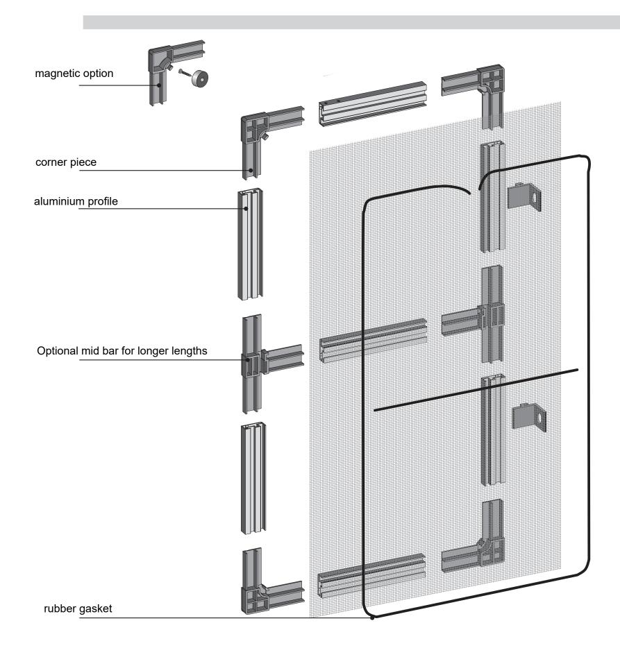
These screens have aluminium frames finished in white polyester coating for ease of cleaning. There are options of having the screens hinged, at the top or sides, magnetic fixings and mid cross bars for adding strength to longer lengths.
