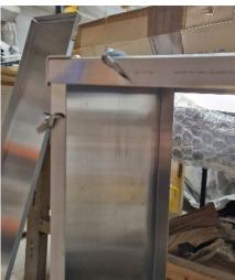
Build the canopy by joining and securing the 4 sections to the angled corner pieces. You will need to use a little force to insert the sections together.
